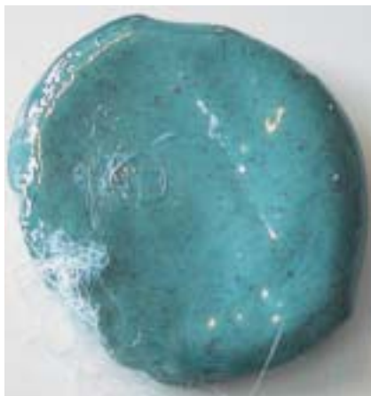
Fig. 3. Organic contaminants and aluminium particles in the flushed compound generated in the process of PET bottle flakes
