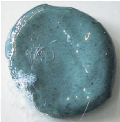
Fig. 5. Organic contaminants and aluminium particles in the backflushed material from processing PET bottle reclaim
